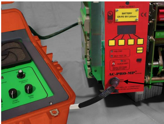
Figure 2 Test Set Connected to AC-PRO-MP (front test port)
